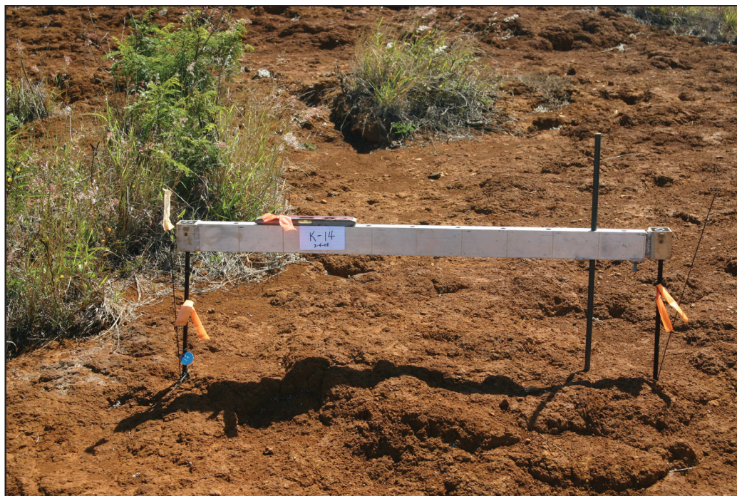
Figure 7. Schematic drawing and photograph of the device used to monitor erosion rates in the Hakioawa and Kaulana watersheds, Kaho'olawe, Hawai'i. (Photographed March 2008 by S.K. Izuka, U.S. Geological Survey.)
